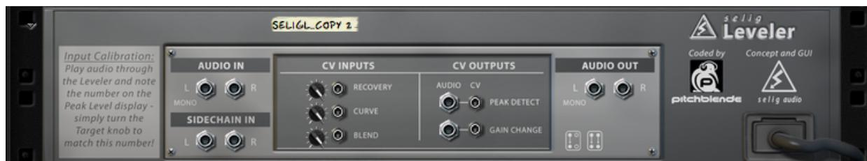
Here you will find all the I/O for the Selig Leveler. Naturally there are audio inputs and outputs, as well as a side chain input. Also included are CV inputs for the Recovery, Curve, and Blend controls, and CV and audio level outputs for the Peak Detector and Gain Change circuits. For easy reference, the calibration instructions are located on the left side of the back panel.
