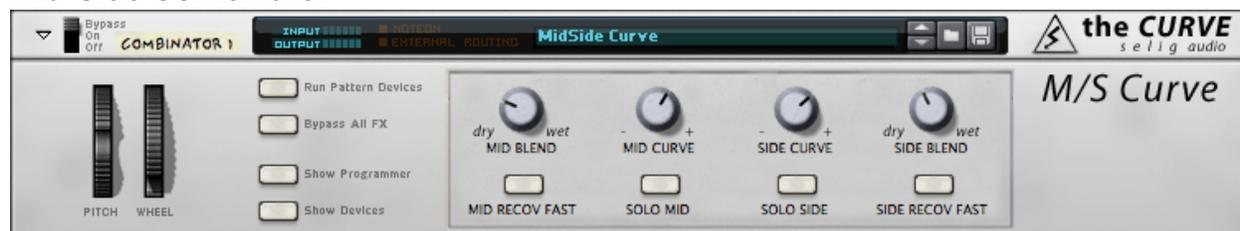
The Mid-Side Combinator allows you to use two Levelers, one for the Mid signal (“Mid Curve”) and one for the Sides (“Side Curve”). This allows you to increase (or decrease) the loudness of either the Mid/mono signal or the Sides signal.
