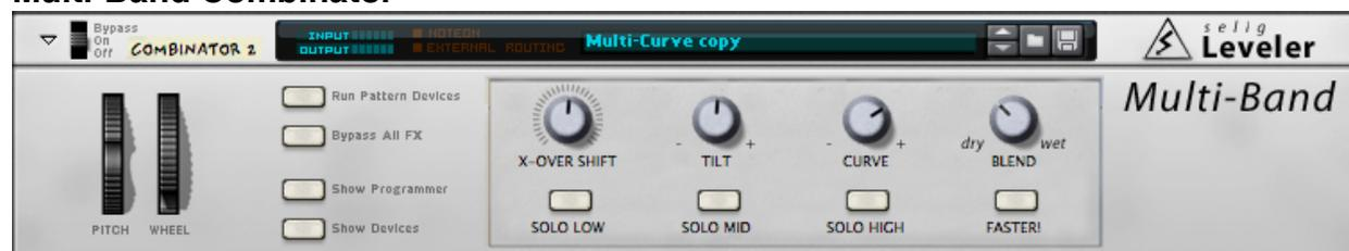
The Multi-Band Combinator is a three band Leveler, suitable for mastering and vocals or anywhere else you would use multi-band dynamics processing.
