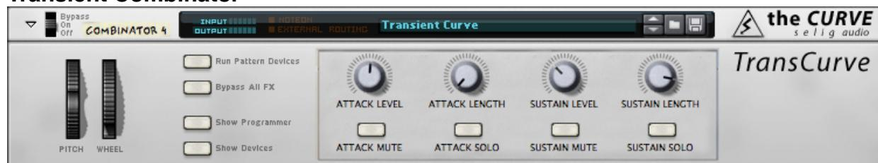
This Combinator uses two Levelers, one for attack and one for sustain. The front panel controls allow boosting attack or sustain (but not cutting). This Combinator is designed to *add* the peak and sustain levels to the original/dry audio signal, and as such will not retain the original peak level of the audio signals it processes.
